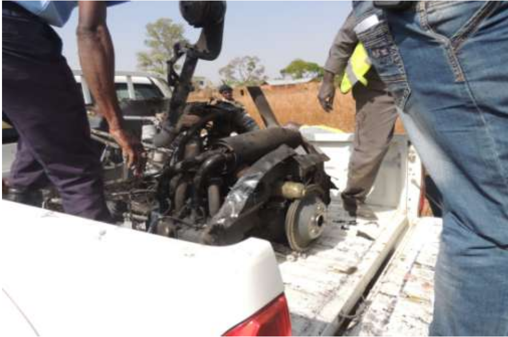
Figure 4: The burnt engine recovered from the aircraft
