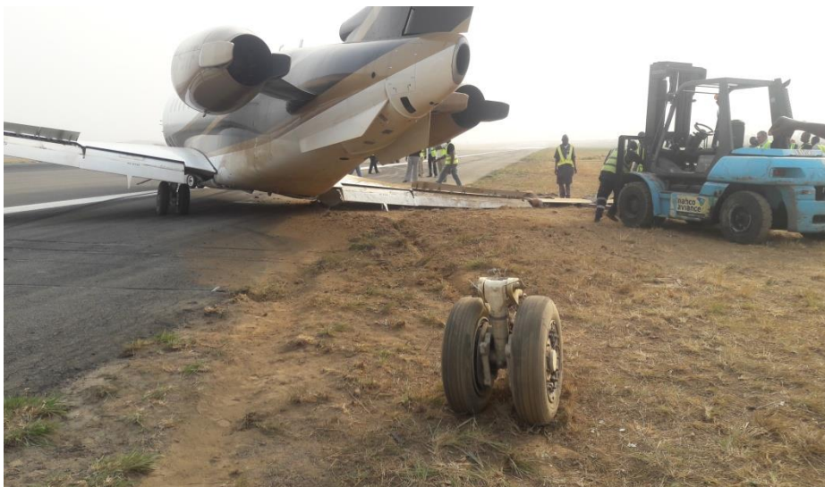
Figure 3: Part of the detached Right Main Landing Gear Assembly
