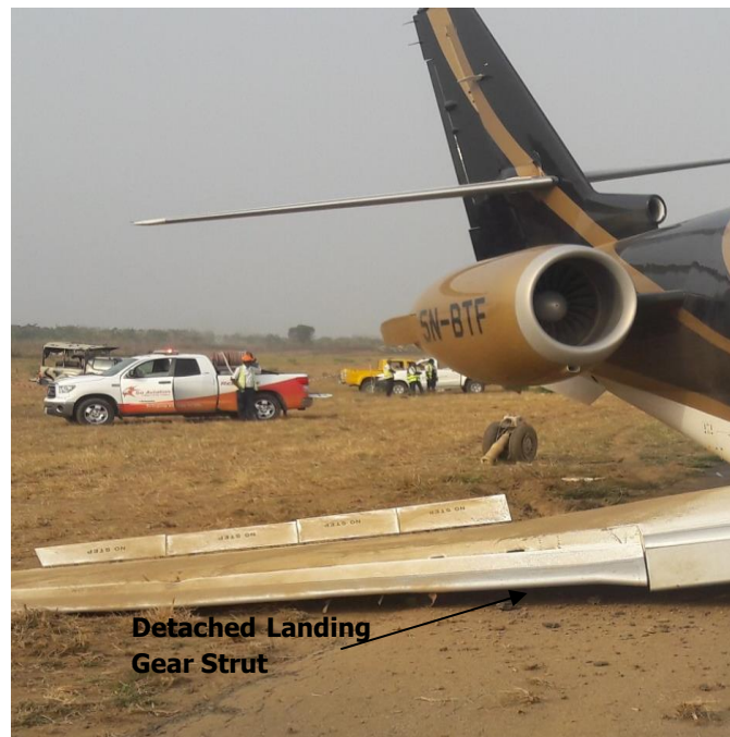
Figure 8: The detached landing gear in relation to the final resting position of the aircraft
